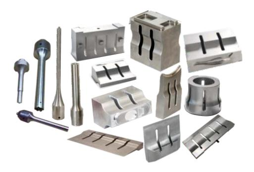
An ultrasonic horn, a sonotrode, is a key component in ultrasonic welding and other ultrasonic applications. It is designed to transmit ultrasonic vibrations from a transducer to a material, facilitating various processes such as welding, cutting, cleaning, and more. The horn amplifies and focuses the ultrasonic energy into the desired material area, ensuring the effective application of the ultrasonic waves.
